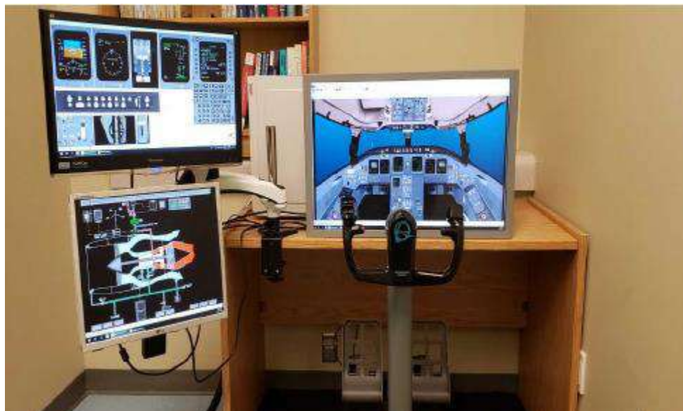
Figure 2. Virtual Research Flight Simulator (VRESIM) for the CRJ-700 Aircraft (developed in collaboration with CAE and Bombardier)
