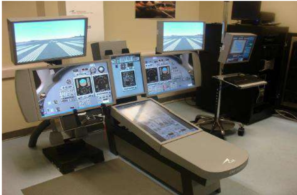
Figure 1. Research Aircraft Flight Simulator (RAFS) for the Cessna Citation X Business Aircraft (developed in collaboration with CAE and Cessna)
